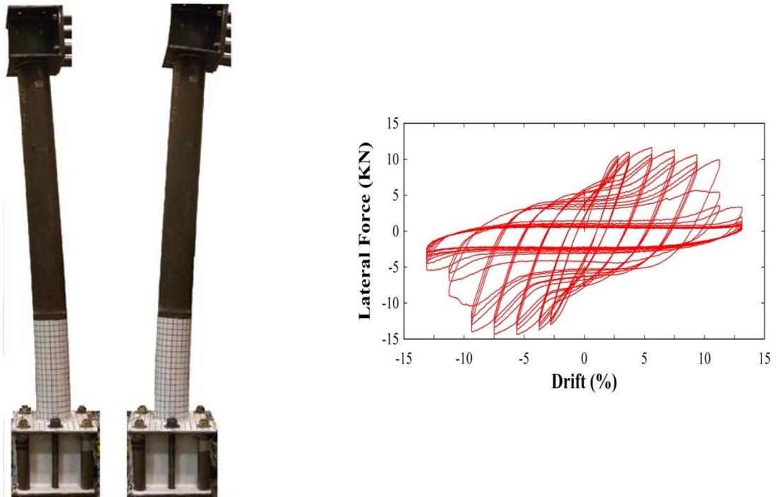
**Figure 8: Specimen at Maximum Strength (Left) and Typical Hysteretic Loop (Right)**
