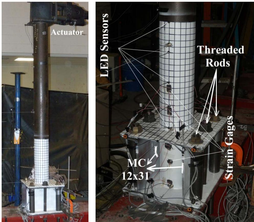
**Figure 4. Cyclic Pushover Test Setup: Global View(Left) and Base Detail (Right)**
