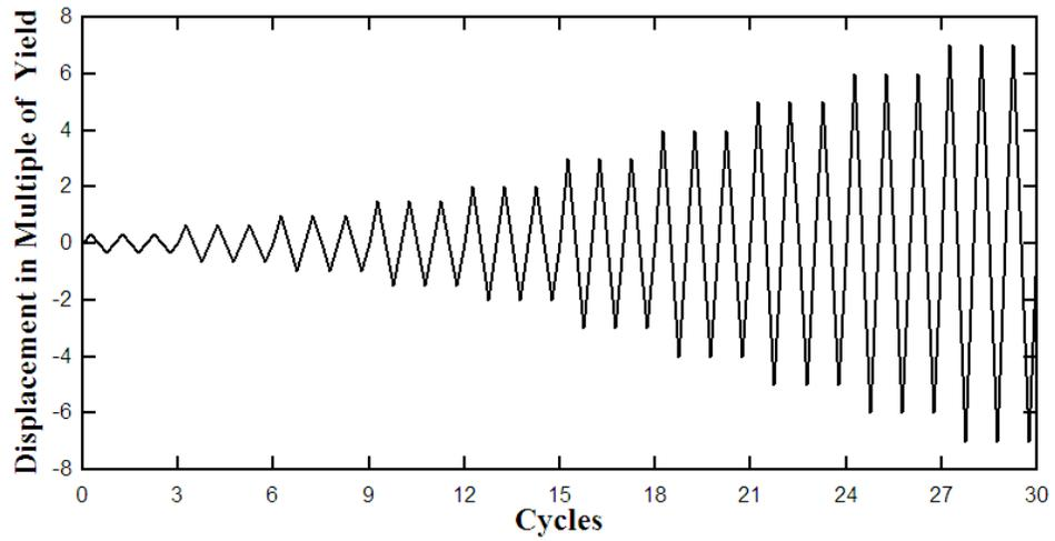
**Figure 5. Cyclic Pushover Test Loading Protocol**
