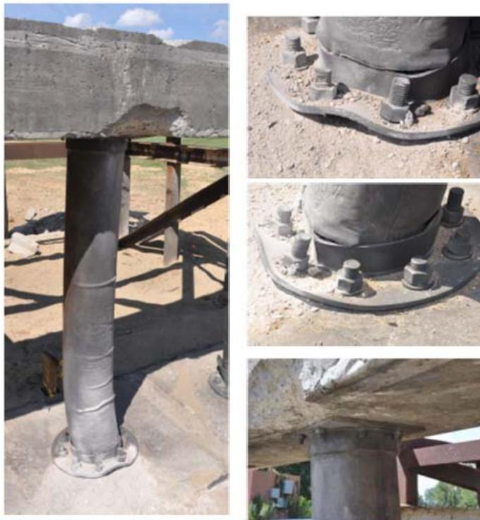
**Figure 7: Global (Left) and Local Deformation (Right) of MSJC after Test**
