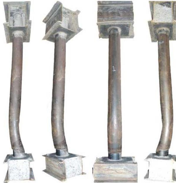
**Figure 6. Plastic Deformation of CFDST under Blast**
