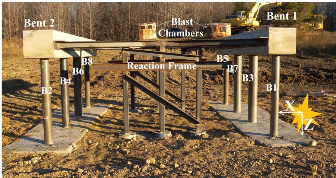
**Figure 3. Test Setup for Blast Experiments**
