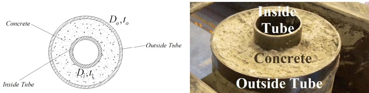
**Figure 1. Concrete Filled Double Skin Tube**
